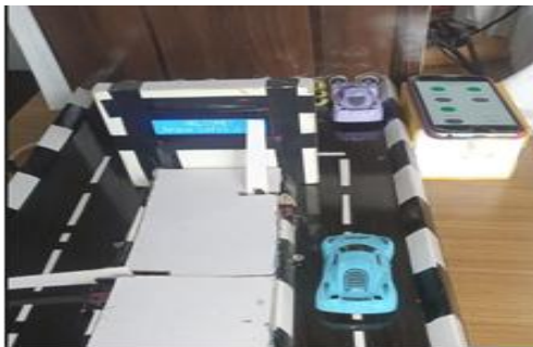
Figure 2: Infrared sensor testing for gate control
